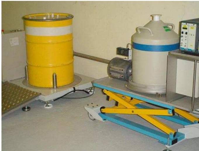
Standard gamma spectrometry device 100 liters WP
